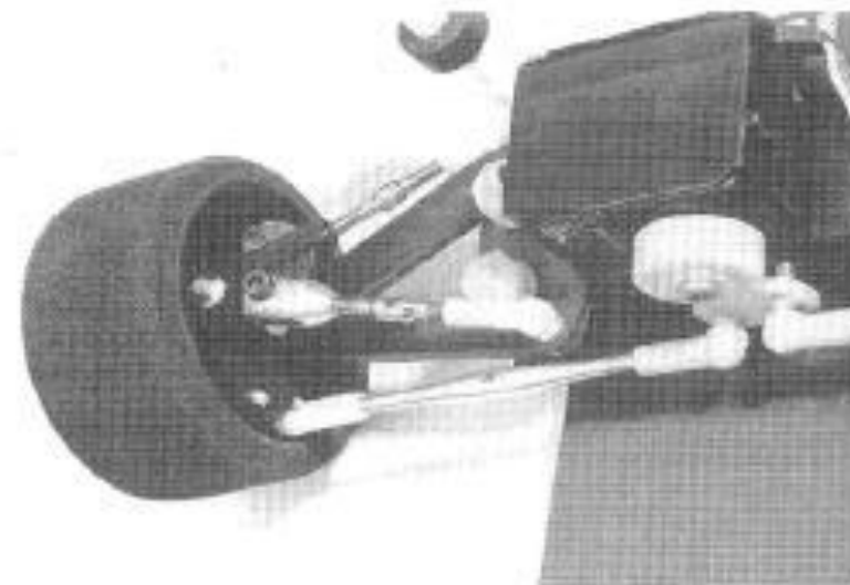
Trinity's Reactive Caster Suspension has a graphite lower arm and fully adjustable upper links that allow for adjustments of caster, camber, damping, spring rate/tension and roll center.
