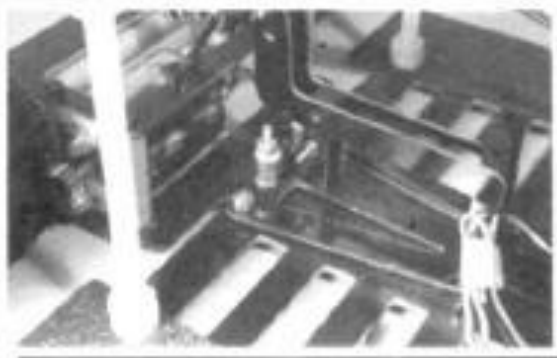
Rear-suspension adjustments can be made both with the coil-over shock assembly and the two tweak/preload adjusters beneath the shock-mount bracket.
