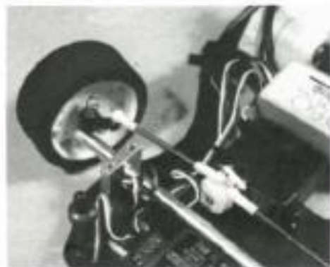
The front end features coil-sprung kingpin suspension and a solid aluminum front axle with adjustable camber.
