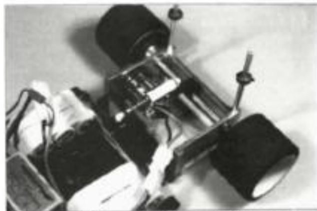
The Outlaw is shown here with a 6-cell saddle pack and a Robart HQ 505 electronic throttle.
