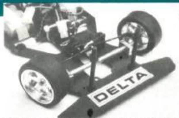
The front suspension is the reliable crossbar design that allows on-the-spot caster adjustment. Note the sharp-locking TMS spoked aluminum wheels and rubber tires.
