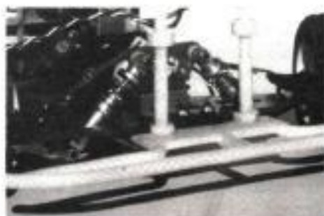
Full view of Invader's independent front suspension.
