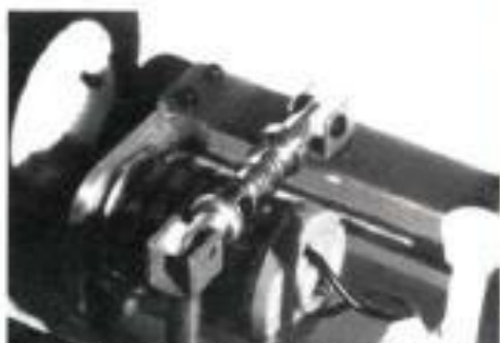
Coil spring on the rear mono shock is fully adjustable.
