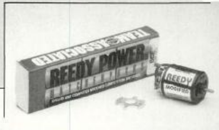
A Yellow-Dot modified motor and a 6-cell SCE Team Pack, both from Reedy, powered the RC10L. A Sassy Chassis motor spacer kept the proper distance between the motor pinion and the spur gear.
