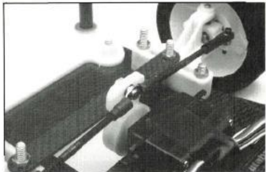
Befry, center-point steering replaced the stock linkages. To clear the linkages, the bolts had to be cut. You won't have to do this if the front ride height isn't changed.
