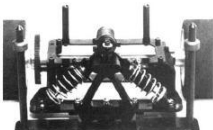
The two short rear shocks control the T-plate twist and roll. The rear body mounts are attached to the main chassis.
